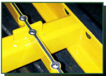
Screen Deck Coated For Abrasion Resistance.
