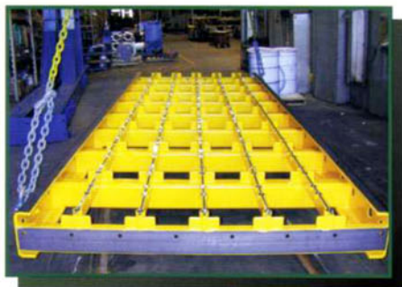
Screen Deck Coated For Abrasion Resistance.
