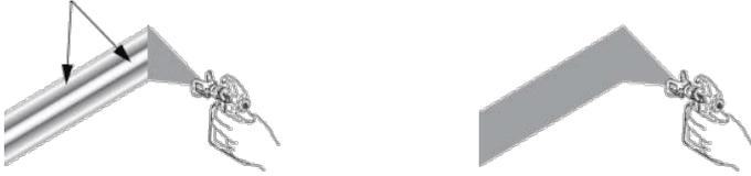
A good spray pattern indicates that the paint or coating is completely atomized and distributed evenly on the surface. Hose length should be appropriate for your machine and always ensure your feed hose is larger than your whip. Having a smaller whip will serve to re-pressurize the coating at the spray gun and assist in correct atomization of the coating.
